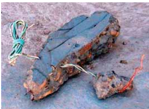
Remote control receiver hidden in plaster.
