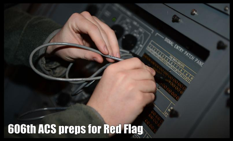
Senior Airman Kodie Hinz, 606th Air Control Squadron data maintenance technician from Goodman, Mo., tests a circuit at the 606th ACS before a live air control mission Jan. 8, 2013. It is crucial to follow checklists and conduct tests to verify that equipment is working properly before each mission.
