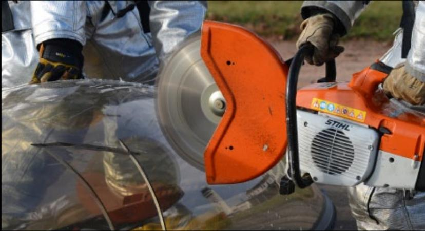
An Airman from the 52nd Civil Engineer Squadron starts a circular saw during emergency egress training outside the Spangdahlem fire station, Jan. 7, 2013. This type of training offers firefighters hands-on experience in cutting through aircraft canopies during emergency egress and pilot rescue situations.
