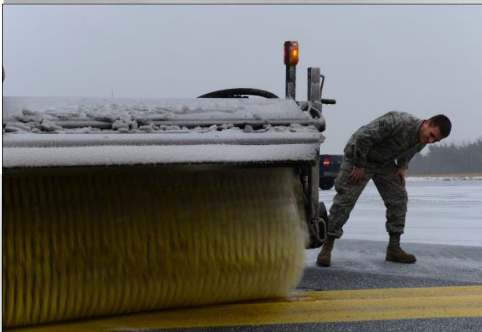
U.S. Air Force Senior Airman Joshua Lemanski, 52nd Civil Engineer Squadron pavement maintenance and heavy equipment operator from Pittsburgh, checks the broom height on a snow broom vehicle Dec. 3, 2012. Lemanski checks the height of the broom to prevent damage to itself and the road surface.
