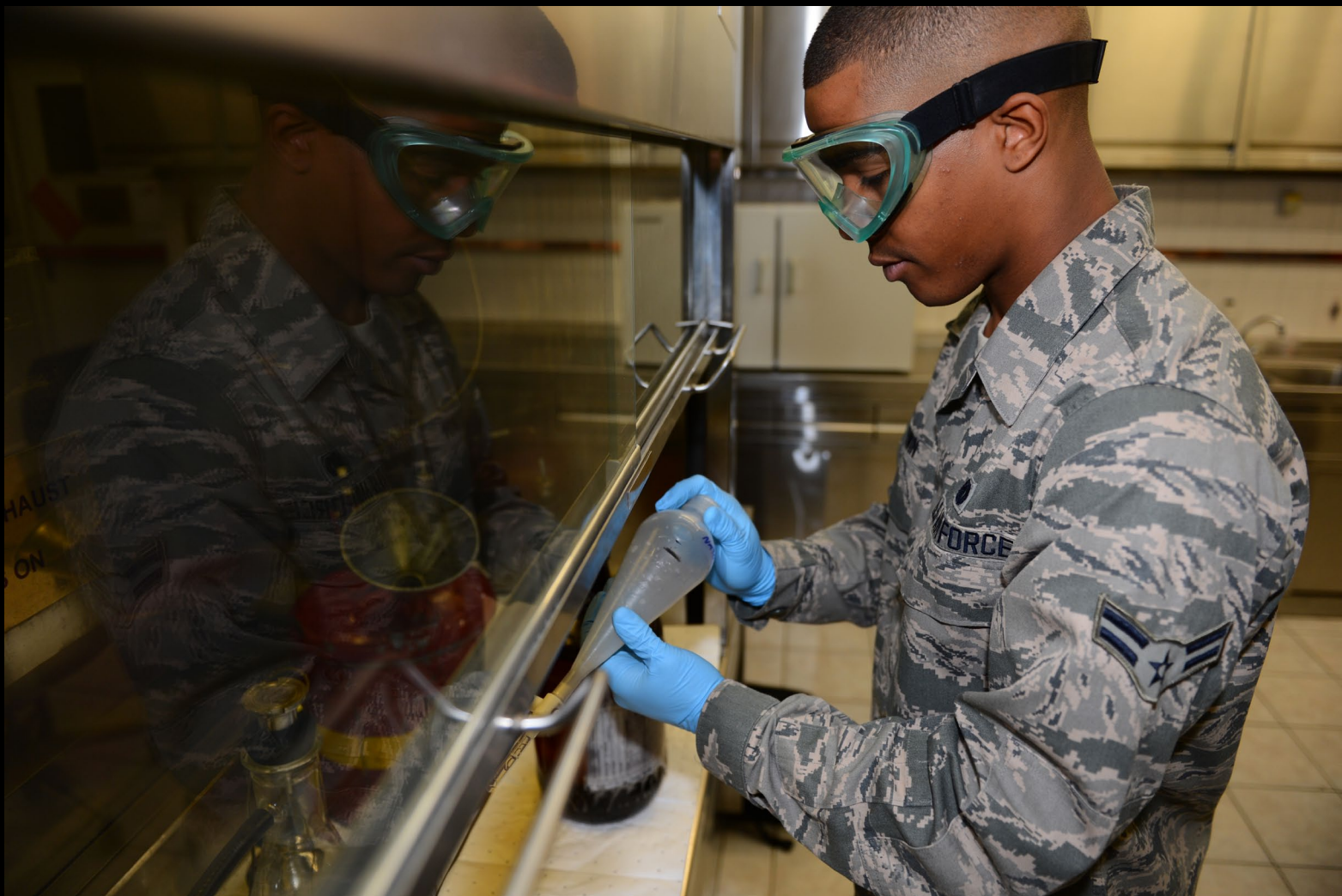
U.S. Air Force Airman 1st Class Anthony Goodwin, 52nd Logistics Readiness Squadron fuels laboratory technician, pours a jet fuel sample into a recycling container inside the fuels laboratory Nov. 7, 2012. The recycled fuel is then reintroduced into the main storage tank for future use. The fuels lab is responsible for testing all petroleum products for use in Air Force aircraft and diesel engine equipment. (U.S. Air Force photo by Airman 1st Class Dillon Davis/Released)
