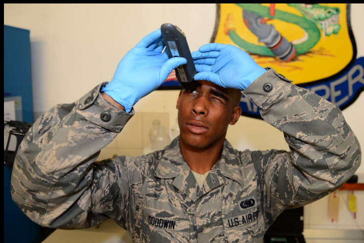
U.S. Air Force Airman 1st Class Anthony Goodwin, 52nd Logistics Readiness Squadron fuels laboratory technician, reads a fuel system icing inhibitor test result using a refractometer inside the fuels laboratory Nov. 7, 2012. The fuels lab ensures that more than 800,000 gallons of jet fuel is properly mixed and free of contaminants before it is used by any Air Force aircraft. (U.S. Air Force photo by Airman 1st Class Dillon Davis/Released)
