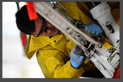
Josh Larkin, 52nd Equipment Maintenance Squadron Fabrication Flight corrosion control civilian contractor, scrubs the landing gear on an F-16 Fighting Falcon in Hangar 3 here May 11.
