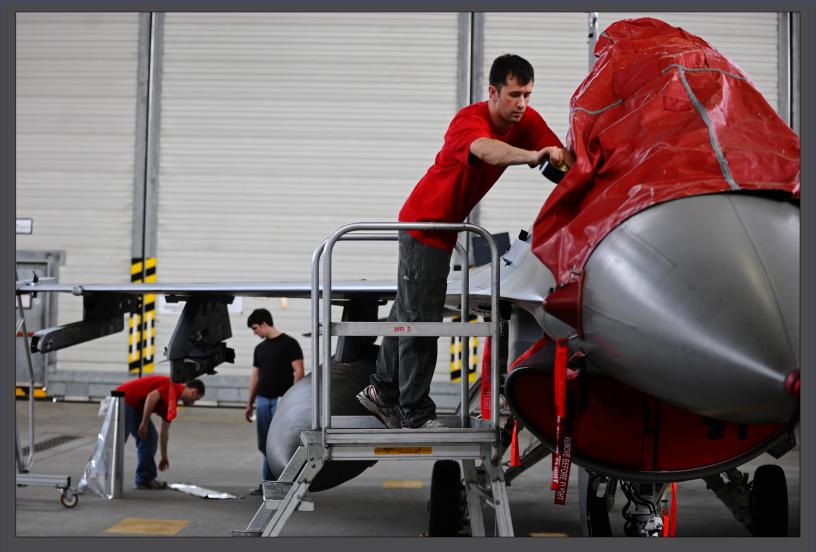
Josh Larkin, 52nd Equipment Maintenance Squadron Fabrication Flight corrosion control civilian contractor, covers the canopy of an F-16 Fighting Falcon before washing it in Hangar 3 here May 11. The fabrication flight contractors wash every 52nd Fighter Wing aircraft twice a year to prevent corrosion and extend the lifespan of the aircraft. For more photos, visit http://www.spangdahlem.af.mil/news/story.asp?id=123301840. (U.S. Air Force photos by Airman 1st Class Matthew B. Fredericks/Released)
