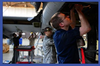
Senior Airman Brandon Spillman, 52nd Aircraft Maintenance Squadron aerospace propulsion journeyman, installs an exhaust on the auxiliary power unit of an A-10 Thunderbolt II during a phase inspection in Hangar 2 here May 4.
