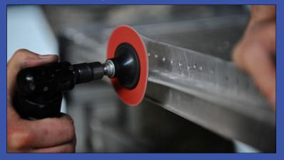
Staff Sgt. Bryan Swift, 52nd Equipment Maintenance Squadron aircraft structural maintenance craftsman, fabricates a fuselage stiffener during a phase inspection in Hangar 2 here May 4. The fuselage stiffener reinforces the panel between the gun-bay and the wheel well.
