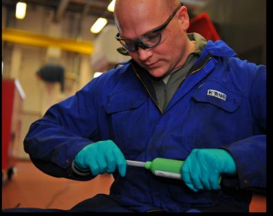
Left: Staff Sgt. Roger Kruback, 52nd Logistics Readiness Squadron vehicle maintenance technician, mixes high-temperature gasket sealant before it can be applied to the surface of a transfer case block during a transfer case rebuild on a P26 Tanker Truck inside the fire truck maintenance shop here Feb. 8.
