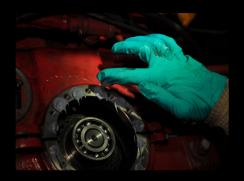
Above: Staff Sgt. Roger Kruback, 52nd Logistics Readiness Squadron vehicle maintenance technician, applies high-temperature gasket sealant to the surface of a transfer case block before the drive shaft can be mounted during a transfer case rebuild on a P26 Tanker Truck inside the fire truck maintenance shop here Feb. 8.
